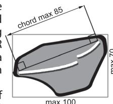
The side dams must be able to contain a square area of minimum 40 mm width and a minimum height of 50 mm to place the car identification numbers".
